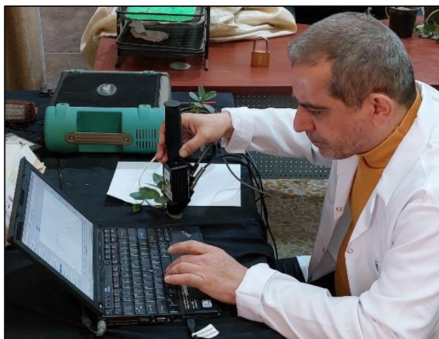
Figure 1. Measurement of the spectral signature of samples using an Analytical Spectral Devices (ASD) device
