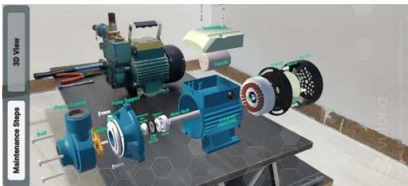
Figure 2. Exploded 3D augmented reality (AR) visualization of the pump assembly for maintenance guidance
