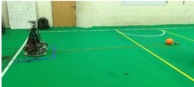
Figure 9. Robot-to-ball distance measurement setup
