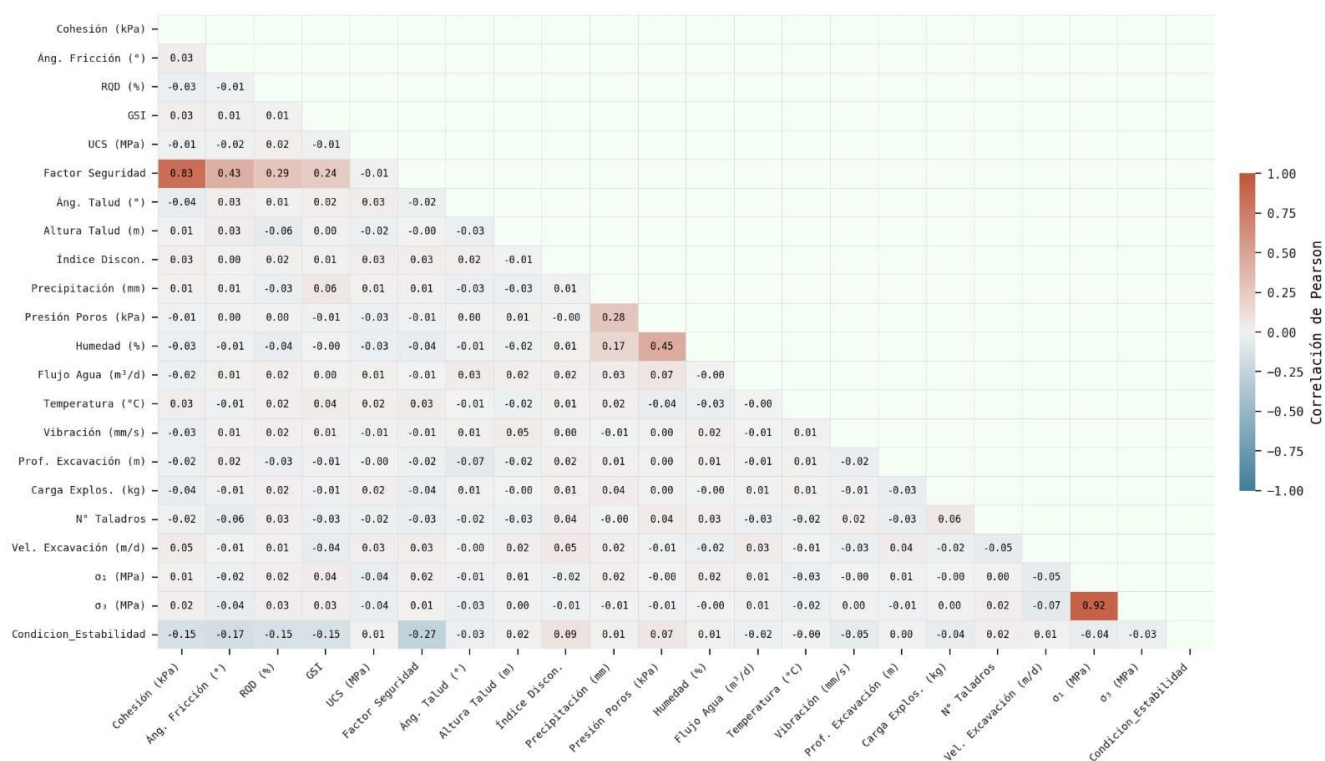
Figure 8. Pearson correlation matrix between the 21 predictor variables and the target variable (stability condition) Note: Red tones: positive correlation; blue tones: negative correlation. The high collinearity between factor of safety–cohesion ( r = 0.83 ) and \sigma_1 – \sigma_3 ( r = 0.92 ), and the moderate association between pore pressure and rock-mass moisture ( r = 0.45 ), stand out.
