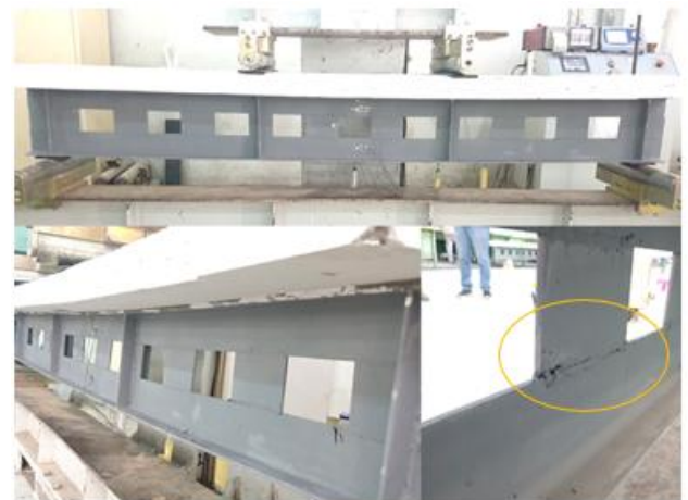
Figure 20. Failure mode of specimen B-1M.50
