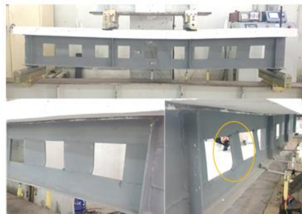
Figure 22. Failure mode of specimen B-1M.70
