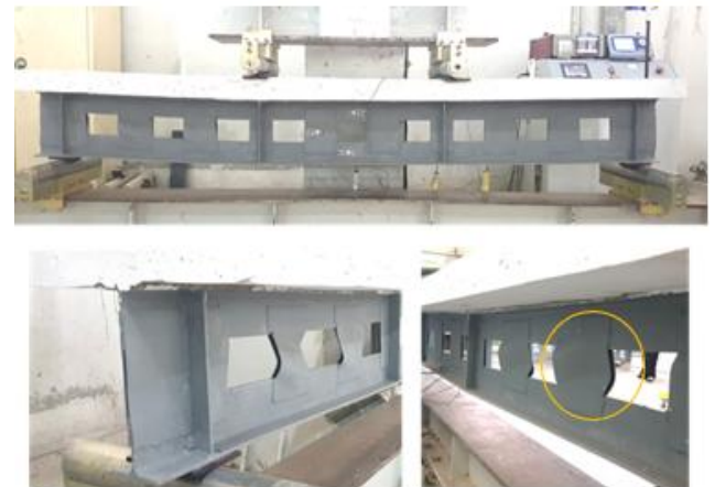
Figure 19. Failure mode of specimen B-2S.50
