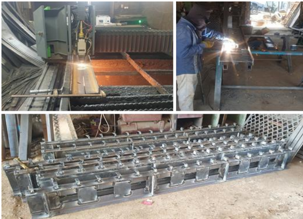
Figure 1. Fabricating process of asymmetric steel profiles
