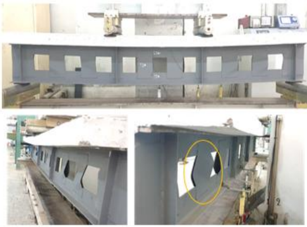
Figure 21. Failure mode of specimen B-2S.70
