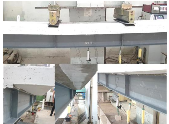
Figure 16. Failure mode of specimen B-NN
