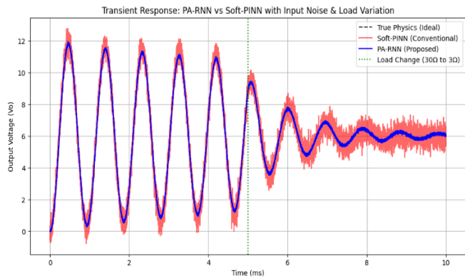
Figure 6. Comparison of transient responses: PA-RNN vs. Soft-PINN with load change 30\ \Omega to 3\ \Omega and 20 dB input noise
