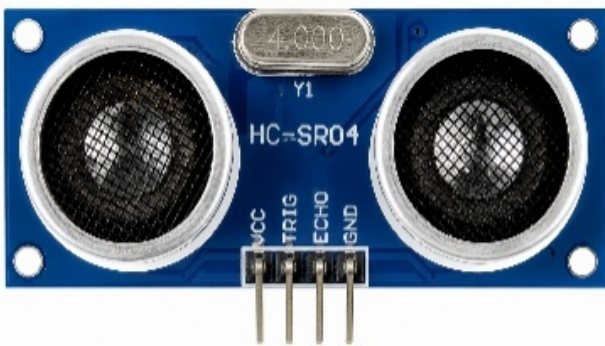
Figure 2. HC-SR04 ultrasonic distance sensor module
