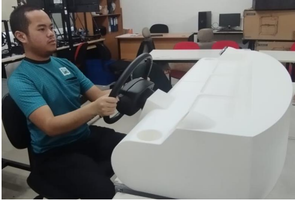
Figure 7. Full-scale 3D-printed dashboard mockup (1:1)
