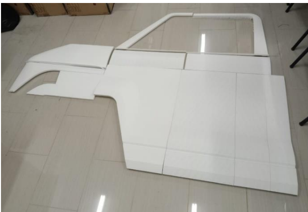
Figure 8. Full-scale 3D-printed door panel mockup (1:1)
