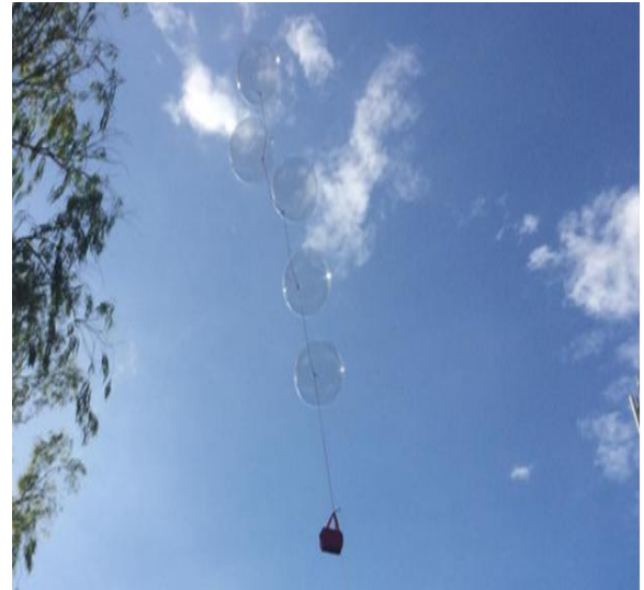
Figure 5. Simulations of multi-balloons with test loads
