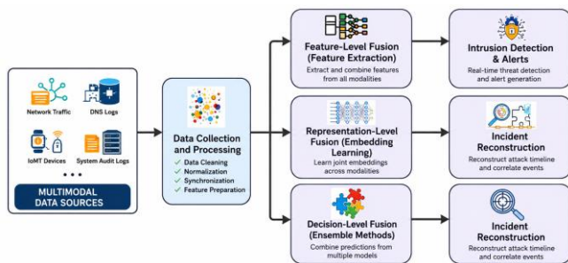
Figure 1. Conceptual pipeline illustrating multimodal data fusion for cyber-forensic analysis in healthcare systems
