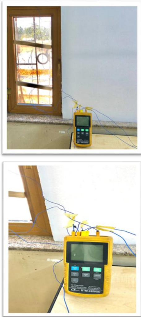
Figure 3. The temperature of the wax was measured using a data logger device
