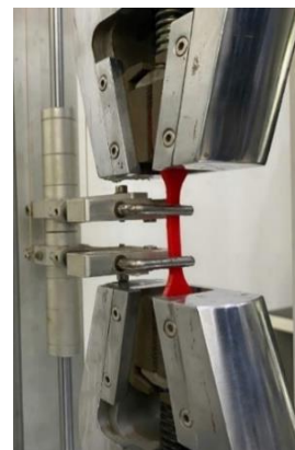
Figure 6. Specimen setup for tensile testing prior to loading
