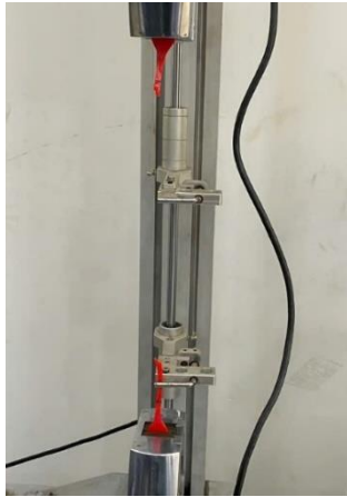
Figure 7. Post-test image of the specimen after uniaxial tensile deformation
