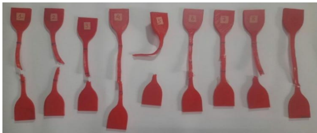
Figure 8. Fractured specimens after tensile testing
