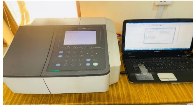
Figure 5. Double-beam UV-Vis spectrophotometer used for optical measurements (Shimadzu UV-1800A, Japan)
