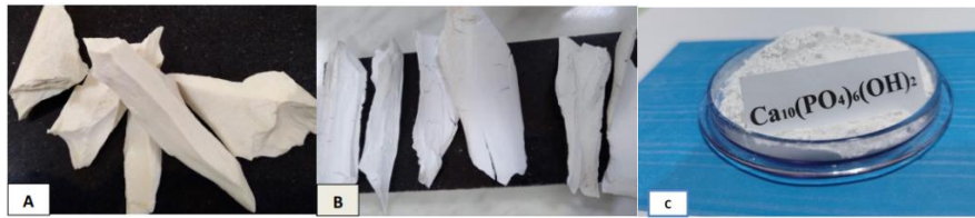
Figure S1. (A) The shape of the bones before heat treatment, (B) The shape of the bones after heat treatment, (C) Hydroxyapatite (HAp) powder prepared in the laboratory
