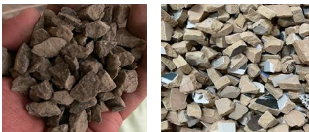
Figure 6. The size of coarse aggregate and ceramic waste aggregate chosen
