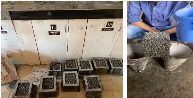
Figure 9. In-house pictures of a pervious concrete cube
