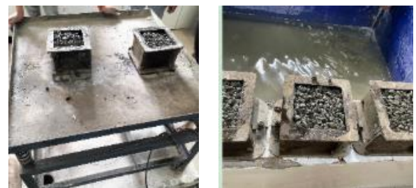
Figure 8. Pervious concrete cube
