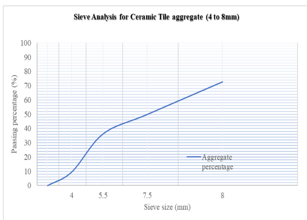
Figure 3. Ceramic tile aggregate sieve analysis (4 mm to 8 mm size range)
