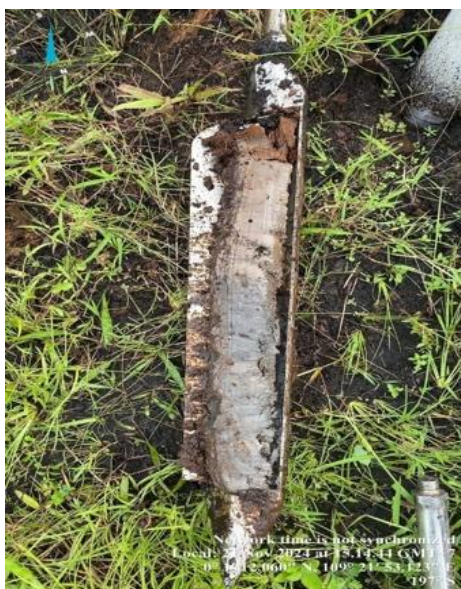
Figure 19. Subsurface profile showing organic-mineral soil stratigraphic boundaries
