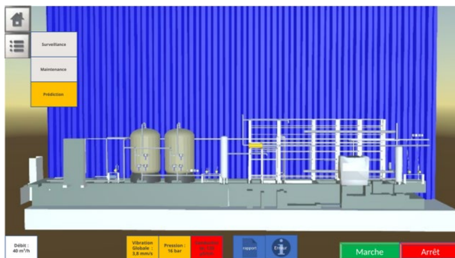
Figure S1. Example of the deployed supervision interface used for reverse osmosis monitoring and decision support
