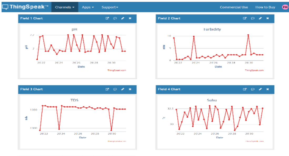
Figure 6. Water quality monitoring graph at Location 2
