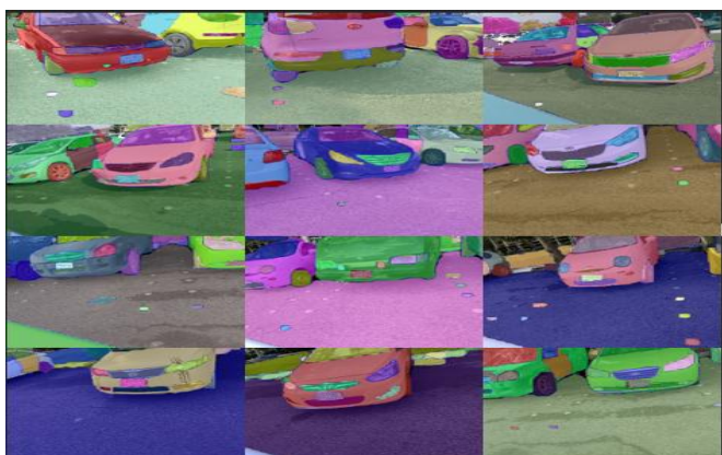
Figure 4. Sample license plate detection results using convolutional neural networks (CNN) + YOLOv8-seg with LAB color space preprocessing
