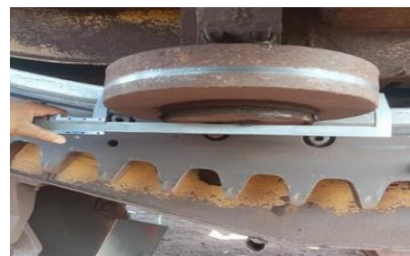
Figure 3. Wear measurement using a caliper
