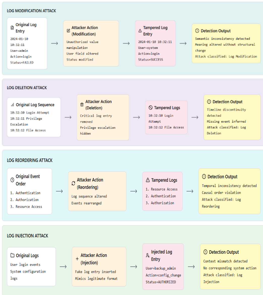
Figure 2. Four types of log tampering attacks: (a) Modification, (b) Deletion, (c) Reordering, (d) Injection
