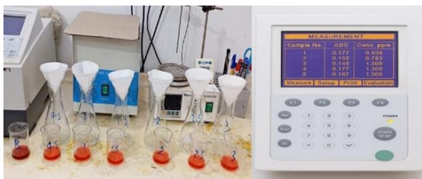
Figure 6. Experimental setup for fluoride ion release measurement using a fluoride ion-selective electrode (ISE), including calibration and sample measurement arrangement
