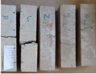
Figure A2. Sample of prisms after bending test after fire
