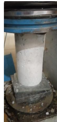
Figure A7. Cylinder sample during compression test
