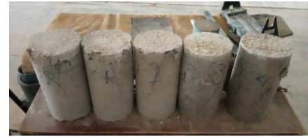
Figure A6. Concrete samples after fire
