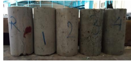
Figure A5. Concrete samples before fire
