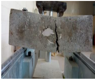
Figure A4. Sample of prisms during bending test after fire
