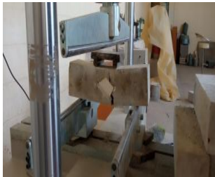
Figure A3. Samples of prisms during bending test after fire
