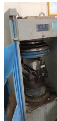
Figure A8. Cylinder sample during tensile test
