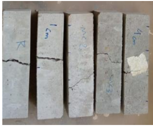
Figure A1. Samples of prisms after bending test after fire
