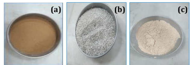
Figure 1. Raw materials used: (a) dune sand (DS); (b) ceramic waste sand (CWS), and (c) limestone filler (L)
