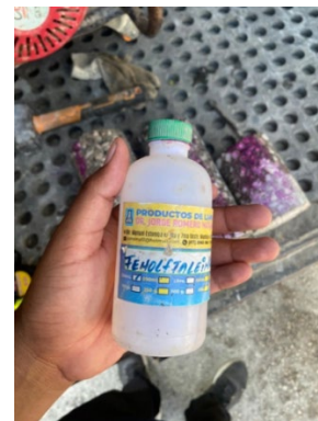
Figure 7. Phenolphthalein solution used for carbonation testing
