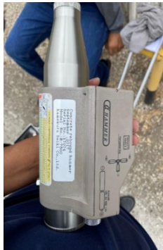
Figure 5. Rebound hammer (Kamekura Seiki Concrete Test Hammer R-7500)
