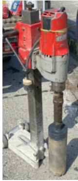
Figure 4. Core extraction equipment (Milwaukee Dymodril)
