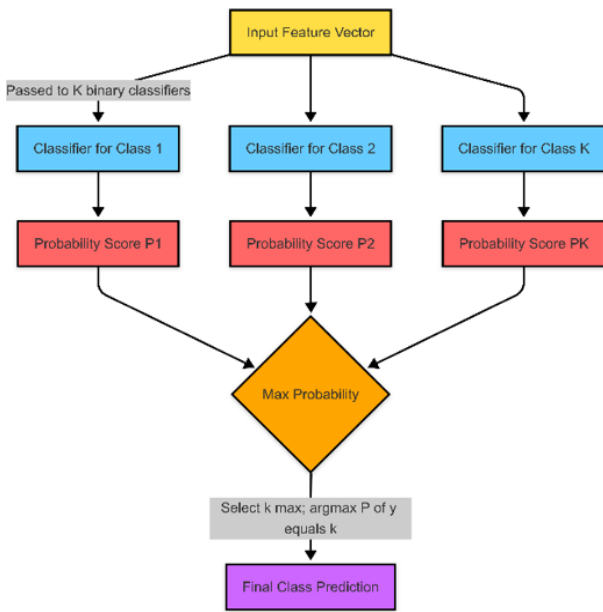
Figure 3. One-vs-Rest (OvR) classification architecture for multi-class prediction
