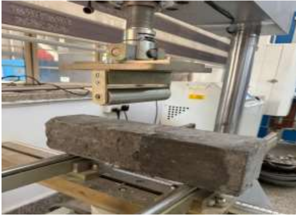
Figure 7. Sample utilized in the flexural strength test
