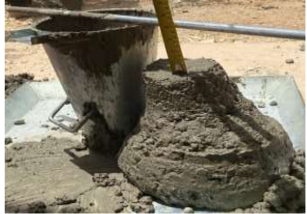
Figure 9. Slump test of polymer concrete
