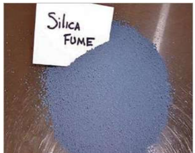
Figure 2. The used ultrafine particles of silica fume
