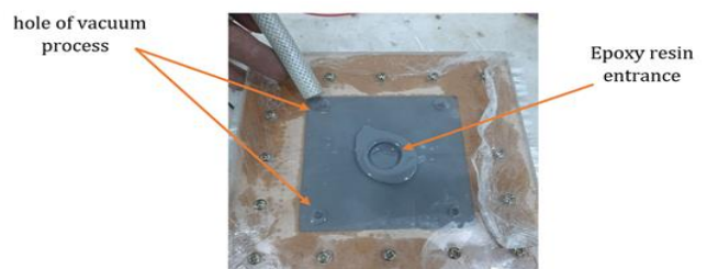
Figure 4. Pouring the resin and the vacuum process
