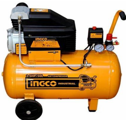
Figure 15. INGCO 50L (AC25508) air compressor
