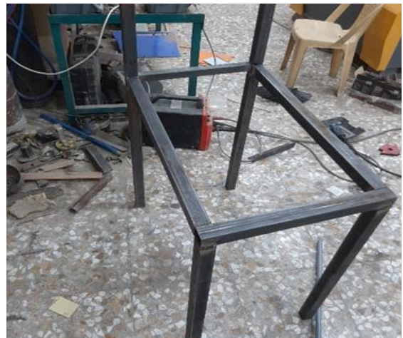
Figure 13. Main frame structure
