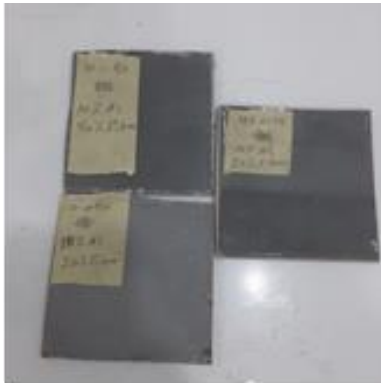
Figure 5. Specimen shields with different fiber orientations
