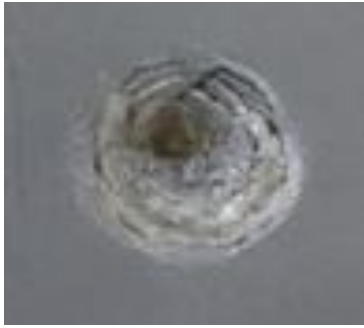
Figure 26. The shape of the experimental deformation area made by the impact shock
