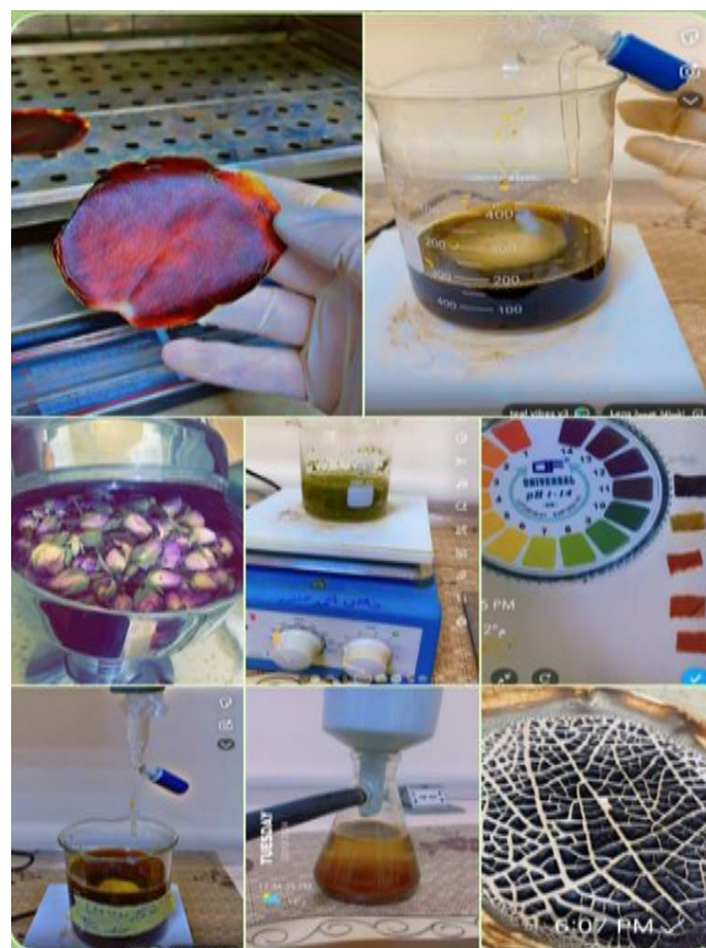
Figure 1. A flowchart depicting the main steps of the plant-mediated synthesis of iron oxide nanoparticles
