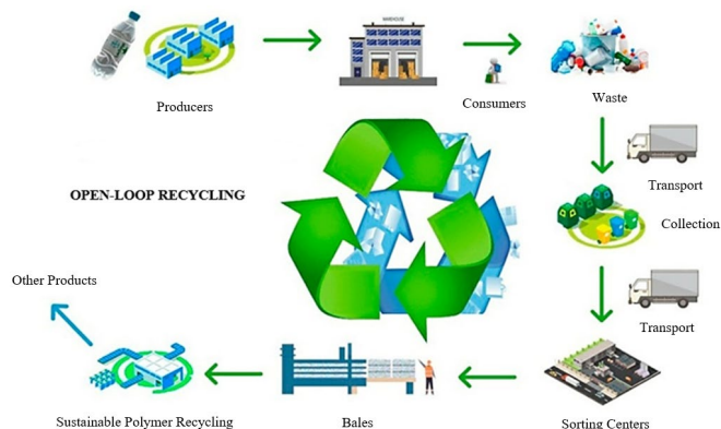
Figure 12. Principle of open-loop (secondary) recycling, where recyclates are typically downcycled into lower-performance applications due to contamination and cumulative degradation [66]
