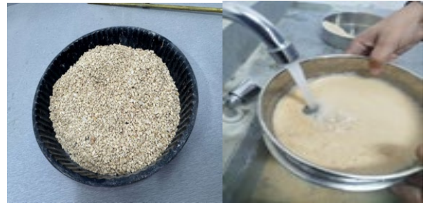
Figure 3. The crushed sand obtained from the crusher waste after the washing process
