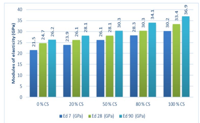
Figure 9. Dynamic elastic modulus with different percentage of crushed sand
