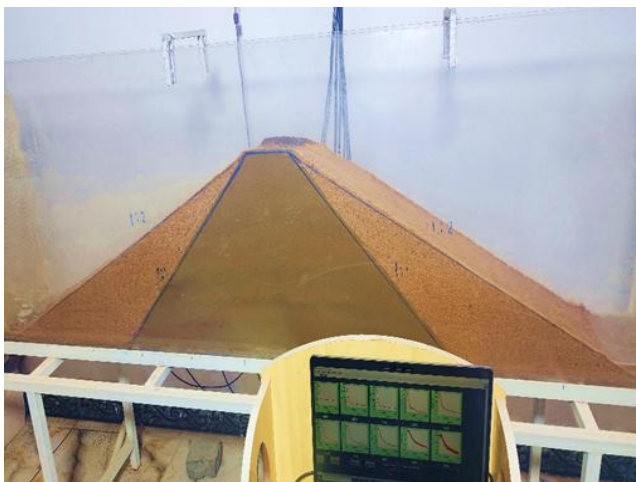
Figure 15. Upstream slope of the M-4 model after rapid drawdown
