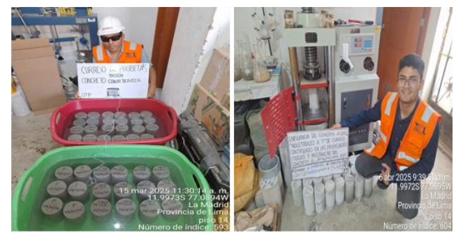
Figure 1. Temperature-controlled concrete curing and compression testing
