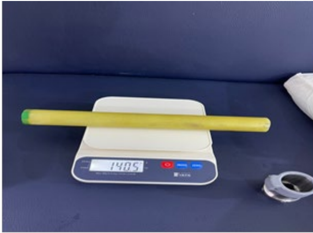
Figure 14. Weight of manufactured pylon
