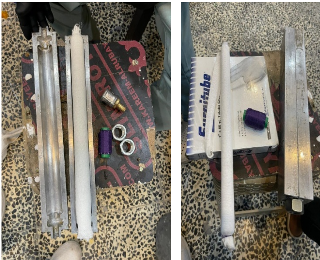
Figure 11. Put glass fibers and Perlon around cylindrical rod
