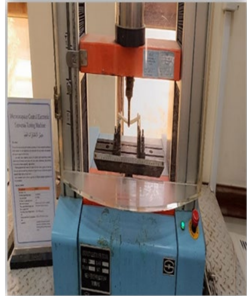
Figure 8. Bending test device with specimen flexural
