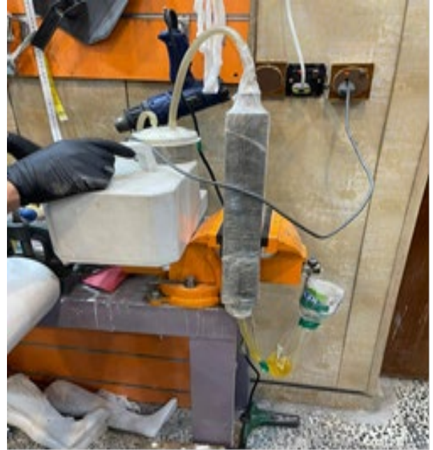
Figure 12. Manufacturing pylons using vacuum bagging technique
