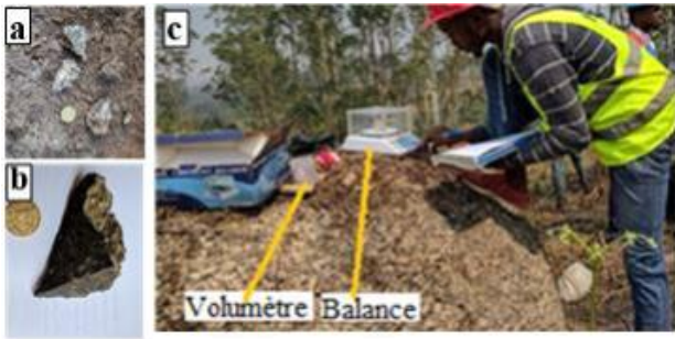
Figure 3. Rock density measurement. a) Granite samples; b) Volcanic rock sample; c) Measuring operation
