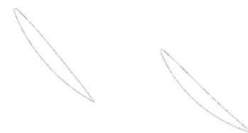
Figure 6. Toroidal foil profile at 0.4 R
