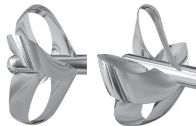
Figure 4. 3D model of toroidal design
