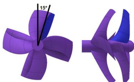
Figure 3. Front and back toroidal propeller design
