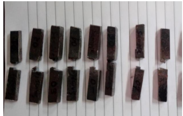
Figure 3. Charpy test samples after the test
