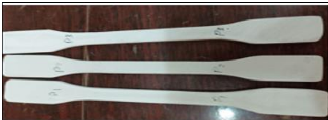
Figure 4. Specimens of the tensile test
