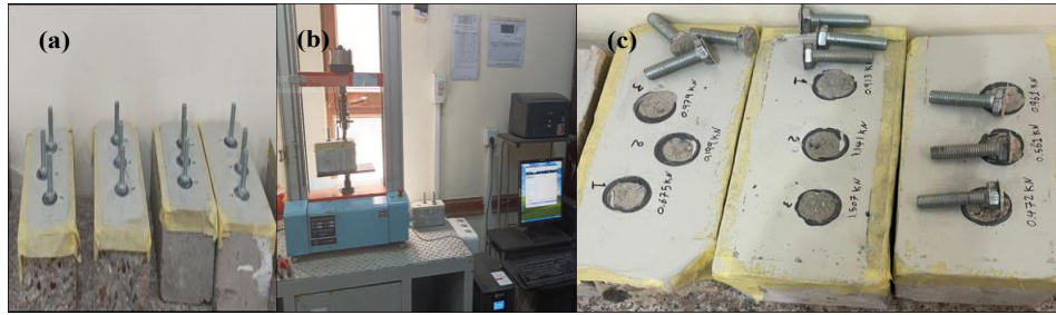
Figure 8. The three stages: (a) preparation of the concrete specimen with bolts, (b) during tensile testing apparatus, and (c) specimens after testing with bolts removed
