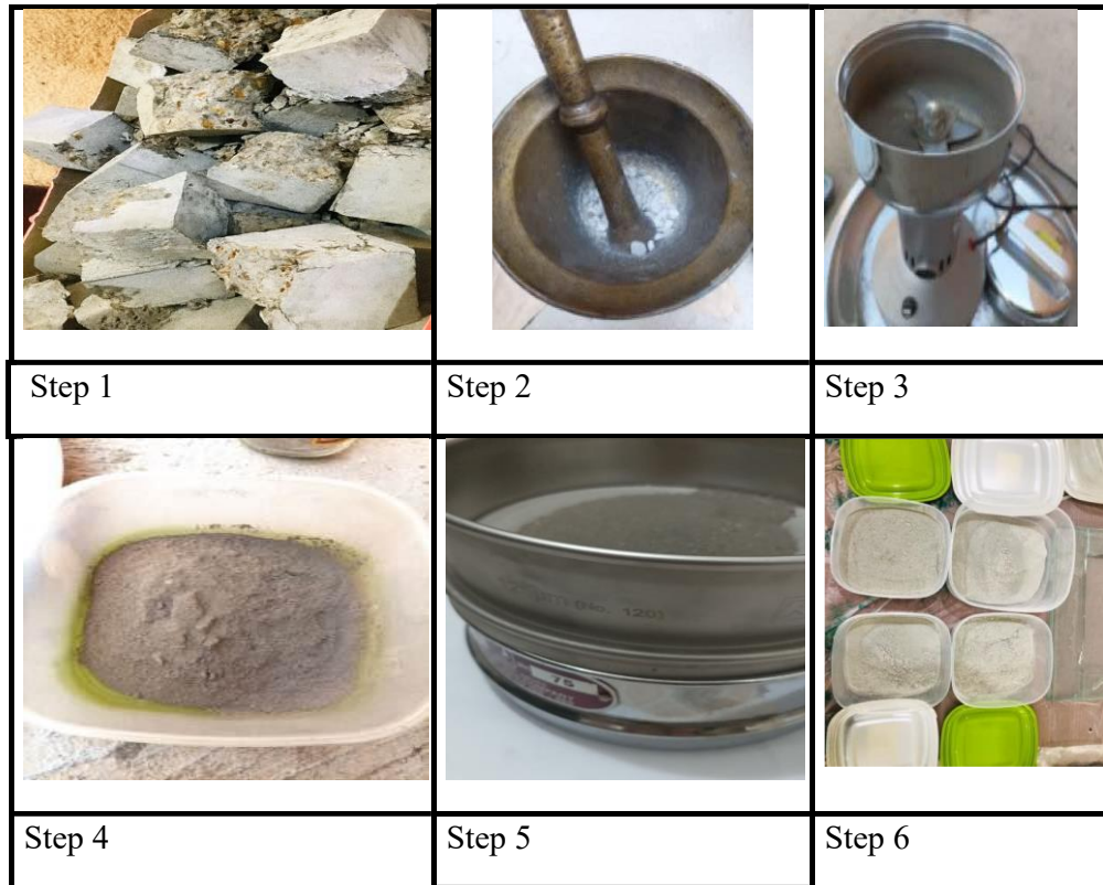
Figure 2. Steps of preparing powder concrete waste
