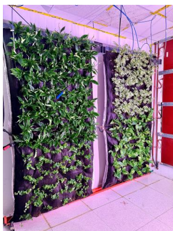
Figure 2. Installed LWs in climate chamber
