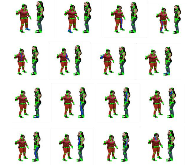
Figure 9. SkeleTrack23 use for relative joint angle feature extraction
