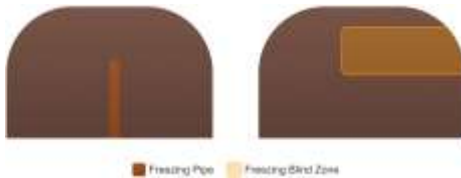
Figure 8. Schematic diagram of positioning defect at the far end of freezing pipe
