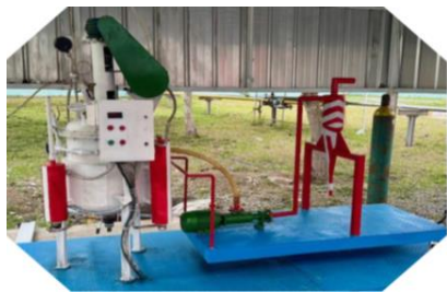
Figure 1. Pilot plant for processing alunite ore with sulfuric acid
