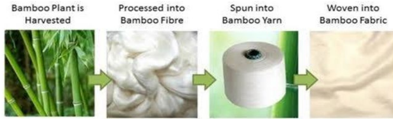
Figure 6. Genuinely processing bamboo fibers in a natural way [22]
