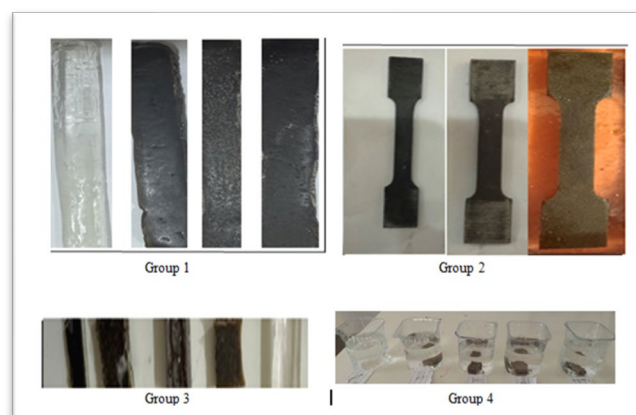
Figure 2. Group 1: membranes of (UP/licorice particles); group 2 and 3: membranes according to ASTM with Mg(OH) 2 ; group 4: all samples immersion with distilled water
