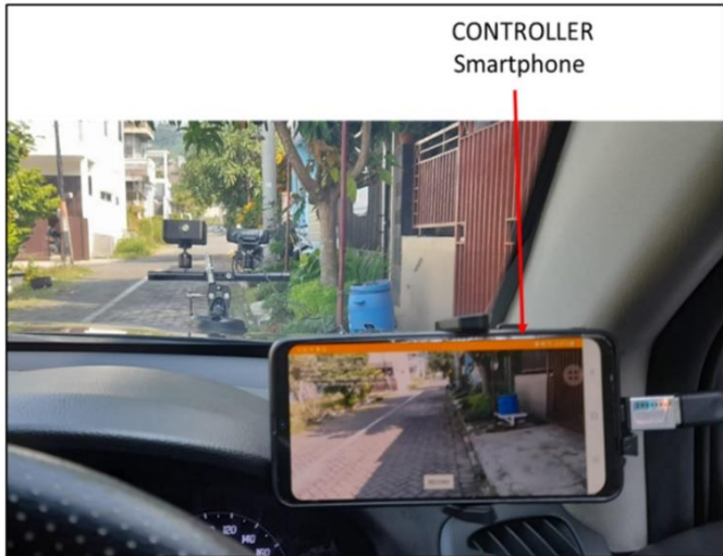
Figure 4. In-vehicle monitoring of external camera feed for road surveying
