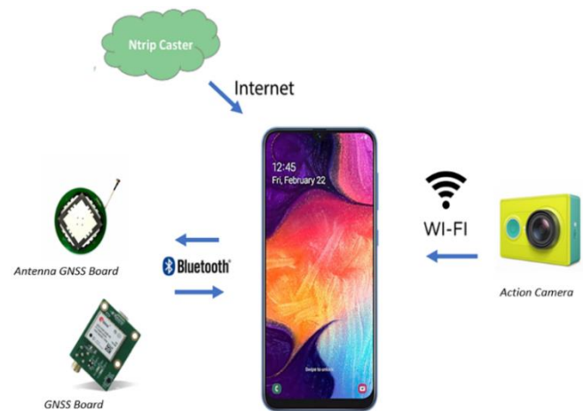
Figure 1. Recording equipment system design
