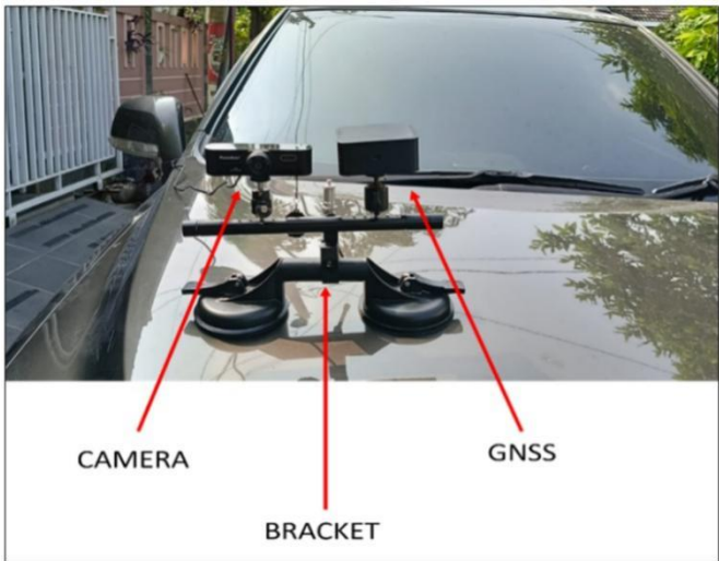
Figure 3. Camera and GNSS receiver configuration on a bracket for road data acquisition
