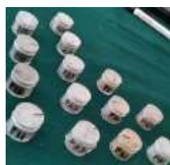
(b) Samples that have been prepared and are ready to measure magnetic susceptibility
