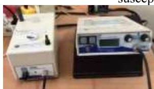
(c) The process of measuring magnetic susceptibility
