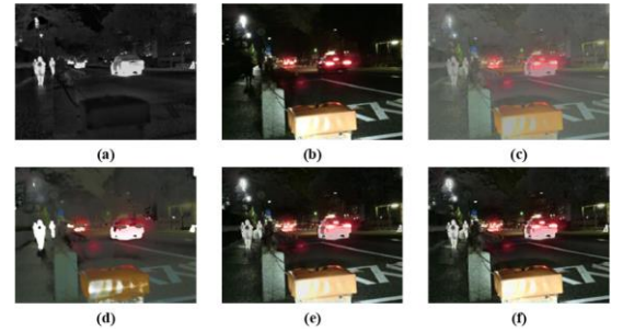
Figure 7. The fusion results of the ablation experiment in the low-light scene. (a) Infrared images; (b) Visible images; (c) Without HAM; (d) Without DCPFM; (e) Without IPR-Net; (f) IPA-Net
