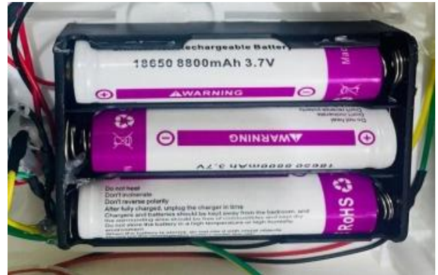
Figure 9. Lithium battery base and battery lithium (3.7 V)
