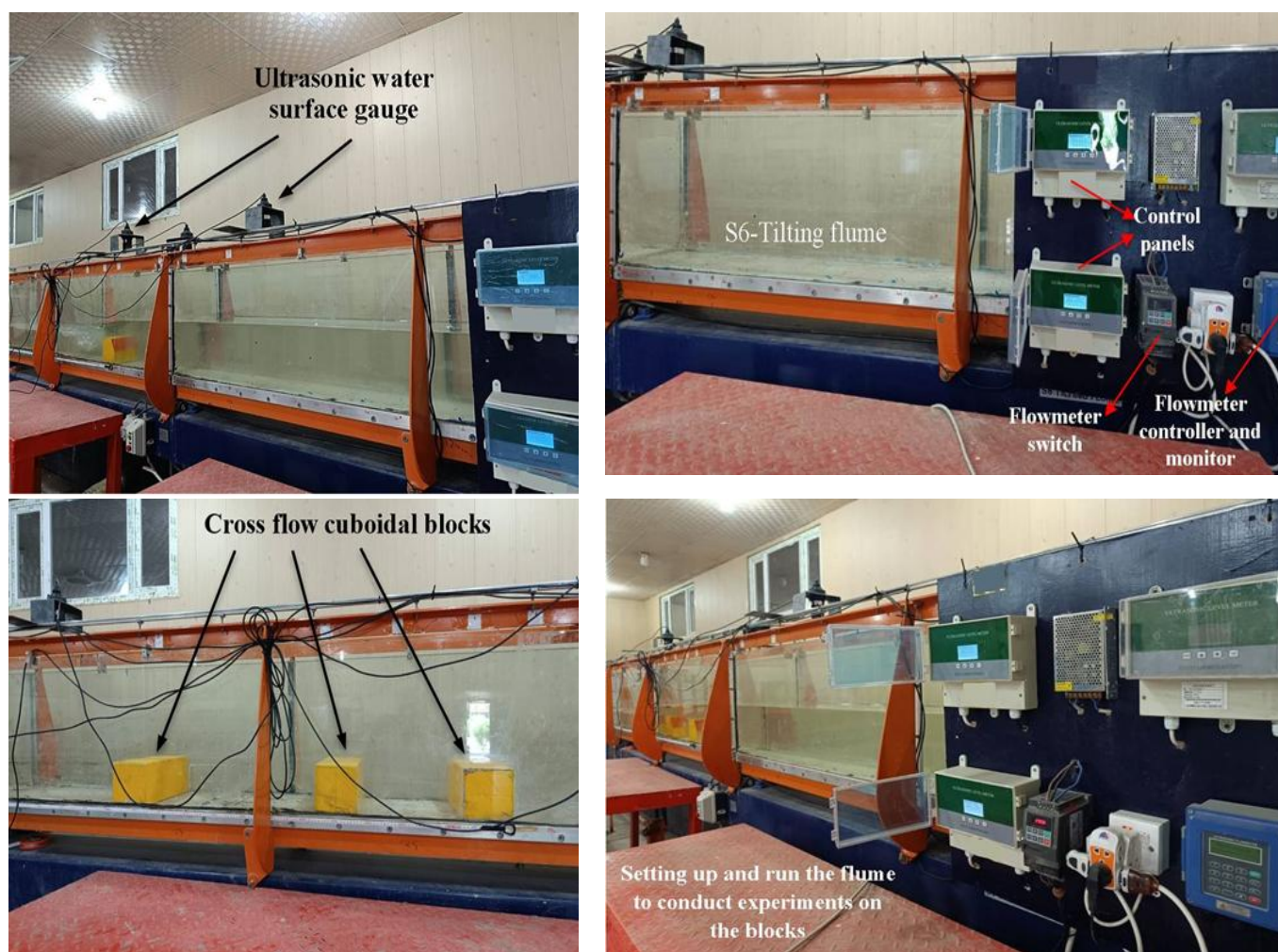
Figure 1. Flume and measurement device setup
