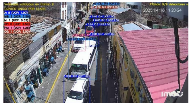
Figure 23. Effectiveness against shadow conditions, showing temporal filtering of false positives
