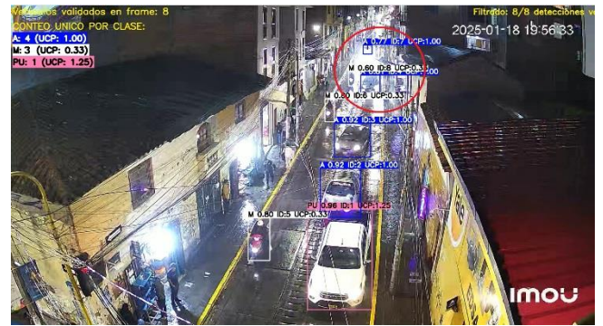
Figure 21. Effectiveness against vehicle light glare and light medium conditions
