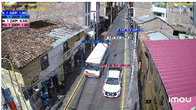
Figure 26. Motorcycle tracking during partial occlusion
