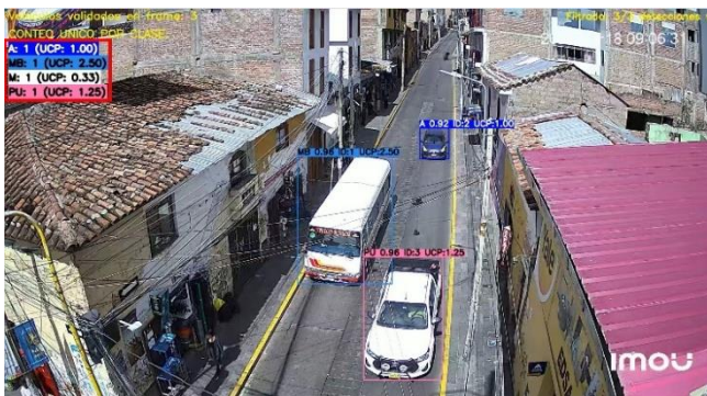
Figure 27. Motorcycle detection loss due to complete occlusion
